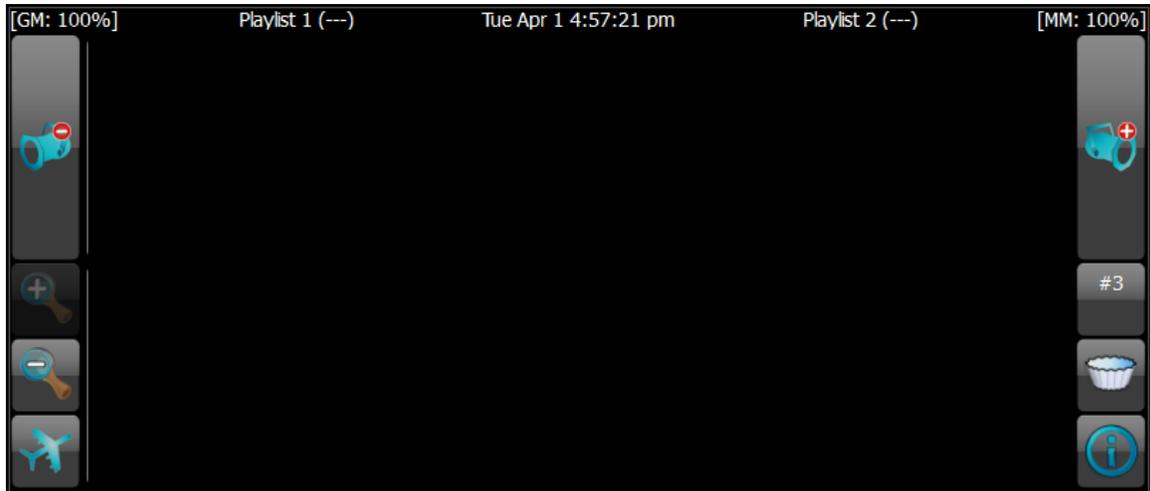
Across the top of the main display is the status bar, which shows the level (in percentage) of the Grand Master and Memory Master; the name of the Playlist currently loaded in each of the right and left playbacks; and the name of the current cue.
