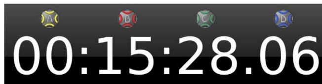
You can quickly zero any of the fields (HH, MM, SS or FF) by pressing the appropriate ABC or D button on the console.
