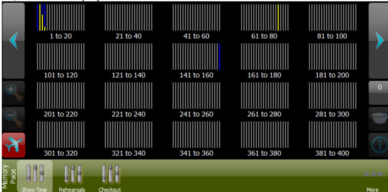
Pressing any bank of 20 will jump you to that bank. Active memories on the old bank will not be released. You may need to “level-match” the sliders to current levels when you switch banks. As always from PLAY MEMORIES, you can be in any bank and press the large left/right arrows. Remember, each Memory Page has 400 possible Memories, but you are not limited to the number of Memory Pages per show file. Add more pages by pressing MORE... then ADD PAGE.
