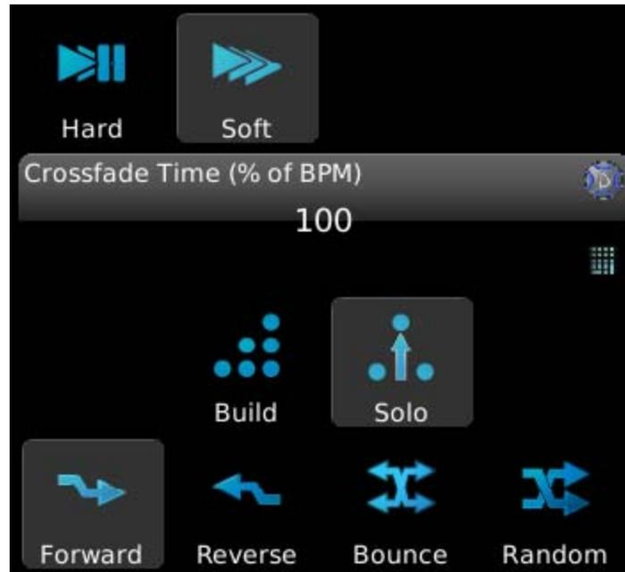
**Direction** - The bottom four buttons change the direction of the chase, either Forward (top down), Reverse (bottom up), Bounce (down then up then down again) or Random. Only one of these options can be selected at any one time. Remember, there is no need to assign Links to any cues. The Direction will take care of figuring out which step comes next in the sequence.
