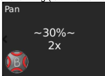
If you hold down the SHIFT button when rolling the wheel, you will change the “X” or number of times the fan is repeated. By default, the entire selection set is fanned from one end to the other. If you SHIFT ROLL the wheel to 2X, you will get two fans, one from one end to the middle of the selection and a second fan from the middle to the end of the selection.
