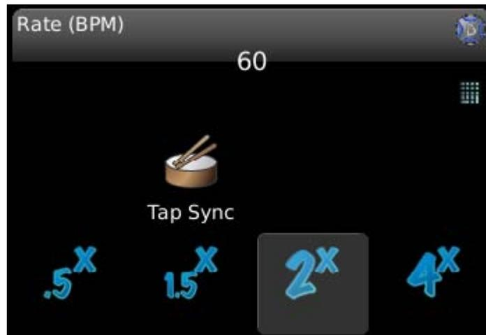
**Rate** - The rate is measured in Beats Per Minute (BPM). So, if the chase is running at 60 BPM, each second will advance to a new step. Roll the blue D wheel to adjust the rate in real time or touch the bubble and type in a specific rate.
