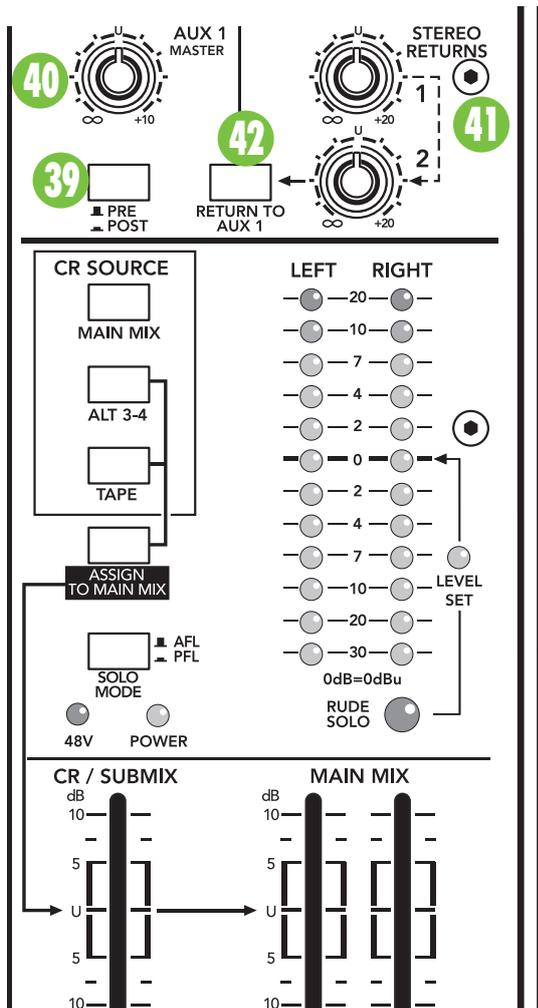
Signals passing through these controls will proceed directly to main mix, with one exception (see paragraph below). The stereo returns do not have mute/alt 3-4 switches, so if you want these signals to get to the alt 3-4 mix, you'll have to patch the effects device's outputs into one of the stereo channels, and mute/alt those channels.
