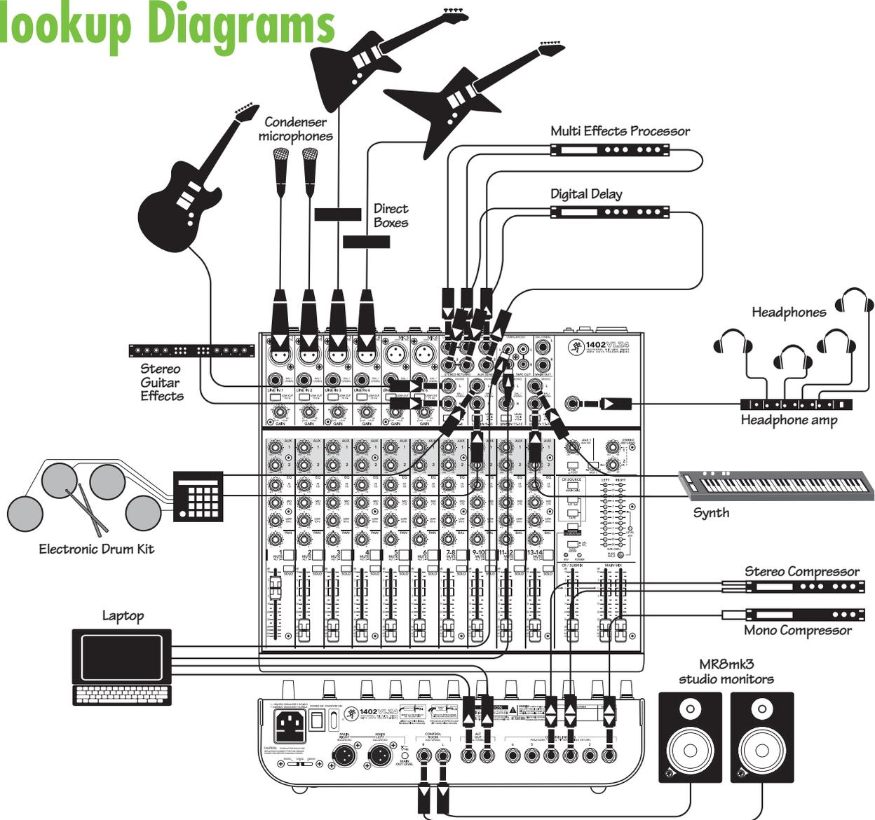
This diagram shows microphones connected to the mic inputs of channels 1 and 2, and a vocal compressor connected to the channel 1 insert jack. Bass and electric guitars are attached to channels 3 and 4 via DI boxes with a stereo compressor on the insert. The lead guitar plays through a stereo effects processor plugged into channels 7 and 8. An electronic drum kit is connected to channels 9 and 10, while a synth is connected to the line inputs of channels 13 and 14.
