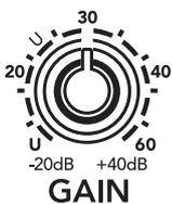
Gain adjusts the input sensitivity of the mic and line inputs connected to channels 1 through 6. This allows signals from the outside world to be adjusted to optimal internal operating levels.
