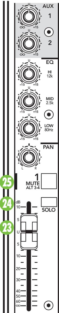
Another way to do the same thing is assign the channels to the alt 3–4 mix, then patch out of the alt 3–4 output back into an unused stereo channel line input. If that’s your choice, don’t ever engage the mute/alt 3–4 switch on that stereo channel, or you’ll have every dog in the neighborhood howling at your feedback loop.
